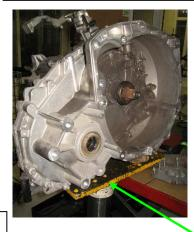
Use the appropriate device to assembly and disassembly the gearbox. The operator never must support the weight of gearbox.
