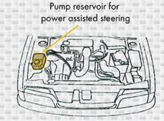
Identification of a vehicle with power assisted steering
