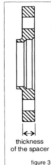
7. Ensure an adequate minimum screwing depth of the supporting thread (see also information in the parts specification and workshop manual).
