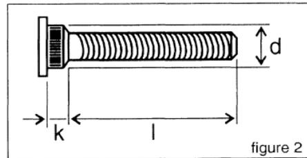
Also make sure that the shaft length of the Eibach special knurled bolts is larger than the original knurled bolts (Figure 3) by the nominal thickness of the spacer.
