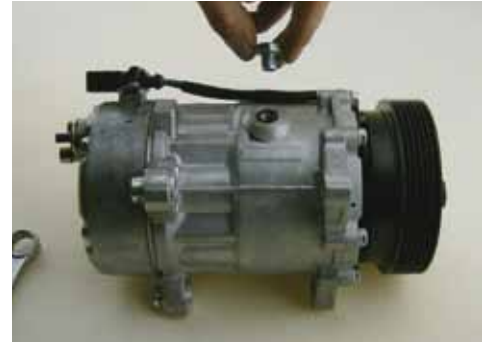
3. Remove drain screw
