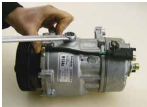
8. Tighten drain screw again
