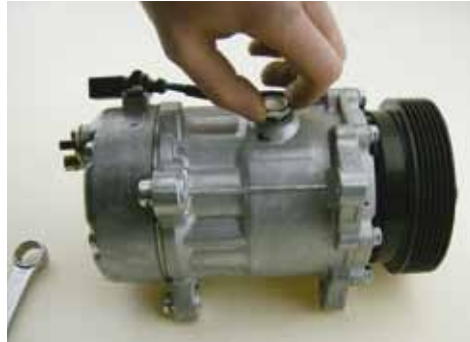
2. Turn out drain screw completely
