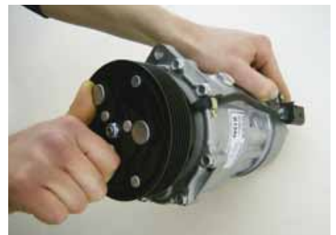
9. Turn clutch 5 times manually to dispose the oil all-over
