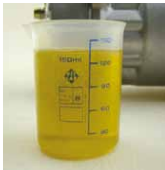
5. Let the oil flow into a measuring jug to state quantity
