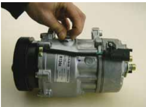
7. Screw in again drain screw with seal
