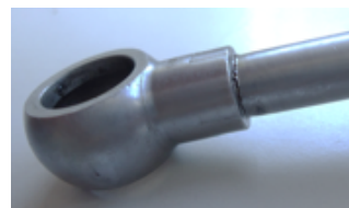
Example of fatigue rupture in the banjo-pipe junction area
